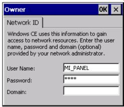
Specific operations must be carried out in order for the selected settings to be retained after a restart. If the entries are acknowledged with OK, the current settings can be saved inside the registry file \NETWORK.REG. The content of the REG file must be inserted in the <a href="Autoexec.reg">Autoexec.reg</a> file so that the settings are reset after a restart.
